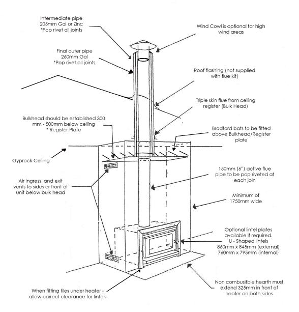
Please note: The Appliance and Flue must be installed in accordance with AS/NZS 2918:2001 and the appropriate requirments of any local building regulatory authority.
